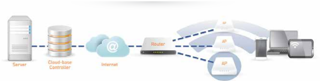
Network infrastructure of cloud-based Wi-Fi controller
