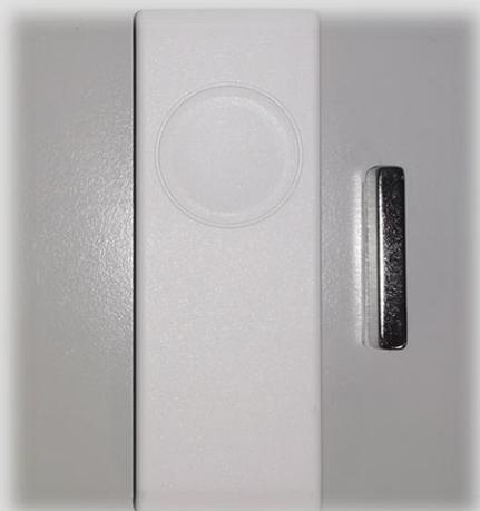
3. The distance between the magnet & device is within 10mm
